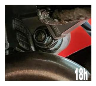
The rubber block on the heat shield should rest on the lower spar of the subframe to assist in damping vibrations. Check that there is no interference of the heat shield with the cylinder head or exhaust headers
