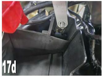
Fit the M6 washers and nuts, but do not tighten yet.
