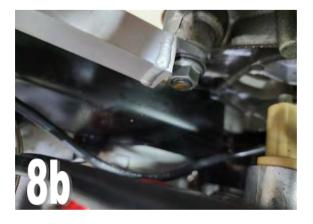
**9)** At this point, fit the rear brake reservoir pot onto it's stay. Just finger tight and really only to keep it up and out of the way.
