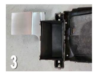
**4)** Also, now is a good time to mount the TYLY-0314X ECU stay. A template for drilling and the necessary mounting hardware is provided with the subframe.
