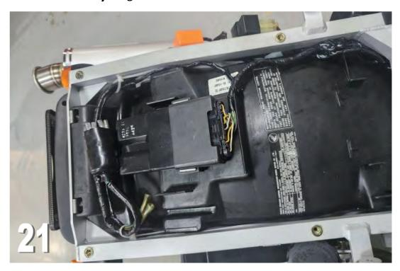
**22)** Now some wire harness management is required. We have provided retained cable ties at four points around the subframe. Use these to tidy up and secure the wires.
