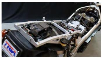
Fitting the TYGA TYLY-0314 subframe is not too difficult. If you managed to remove the standard subframe with ease then the fitting of the TYGA subframe is almost a reversal of that procedure, as we have tried to keep all the components in close to their original position.
