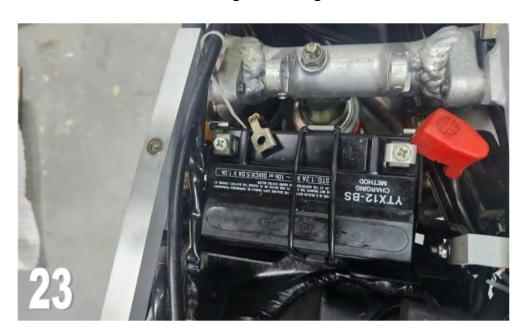
**24)** Due to the compact design, the positive terminal in the wire harness no longer reaches around to the front of the battery positive terminal, so we have made BPSY-0359A Battery Terminal Clip that clips onto the top of the positive terminal of the battery and allows for fitment of the terminal from the side.
