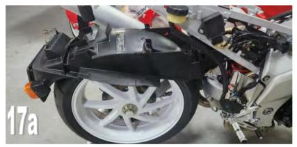
Then you need to lift the front of the undertray up and hook it between the subframe lower left and right spars. The plastic mounts on the undertray are wider than the spars so it takes a bit of a force, pay attention to the heat shield moving into position as it is a tight fit, but it will go through. It is a good idea to protect sharp edges with some painter's tape to avoid scratches.
