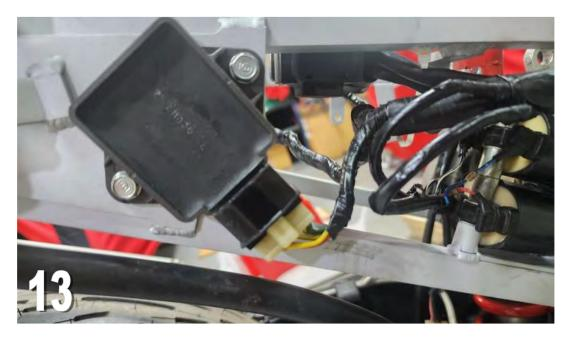
**14)** Plug the starter relay onto the tabs. Note that all the all the wires are running on the outside of the undertray mounting stay at this point.
