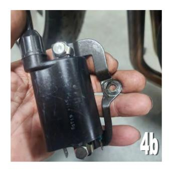
First fit the coil stay to the bike as shown using the bolt that holds the coolant pipe. Just nip this up as we'll need to wriggle the coil around a little to get clearance from the cowling as a final attack. Refit the ground terminal.
