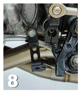
All the left side stays are now fitted. At this stage it is a good idea to fit the choke cable.
