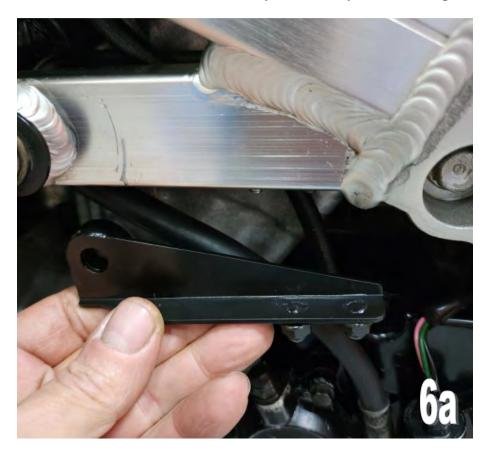
Set the bottom edge of the stay roughly parallel with the frame rail and nip up the engine bolt finger tight.
