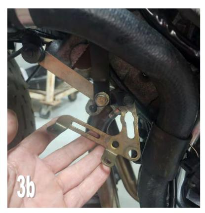
Now you can fit the coolant tank. Make sure to locate the pegs on the bottom of the tank in the holes on the stay, The top mounting tab of the tank should line up with the M6 clip on the top of the stay.
