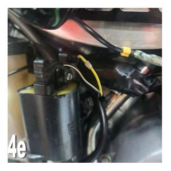
**5)** Now we should do a little wire management to tidy things up. Note the reusable cable tie in use from the salvaged parts. This plugs into a hole on the underside of the frame and keeps things nicely located.
