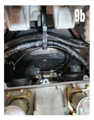
Now fit the choke knob into the stay and screw up the nut. Just finger tight as we may need to modify the position later.
