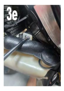
The coolant blow off hose from the radiator passes along the front top edge of the radiator and then through the radiator stay, down the frame rail and plugs onto the bottom spigot of the tank, and the breather hose plugs onto the top spigot and then runs down behind the tank and along the underside of the engine.
