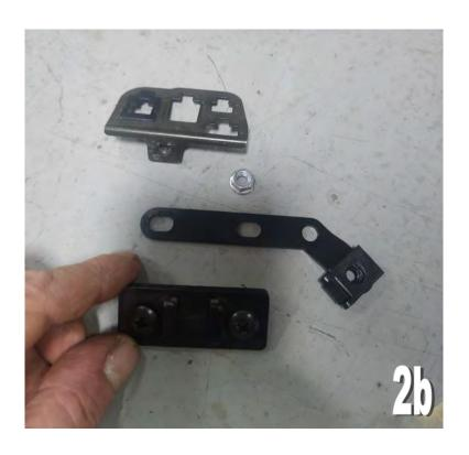
Next, fit BPSY-0353 Stay, Infill/Choke as shown. Fit loosely.
