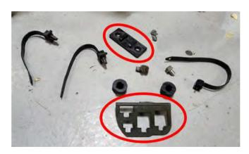
When fitting the stays for the first time, we advise to fit them loosely, as many of the stays have adjustability and will need some fine adjustments when also fitting the bodywork for the first time.
