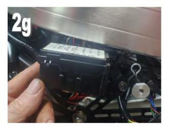
And then we can connect the headlight connectors, pull over the rubber boot and cable tie it to the stay. Check the connection of the running light wire, and tie it all up neatly.
