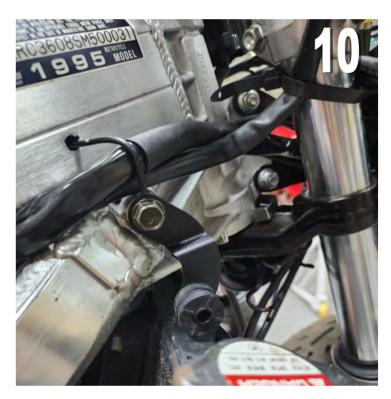
At this point, it is a good idea just to check the movement of the front end to make sure that all the wires run freely and nothing is interfering
