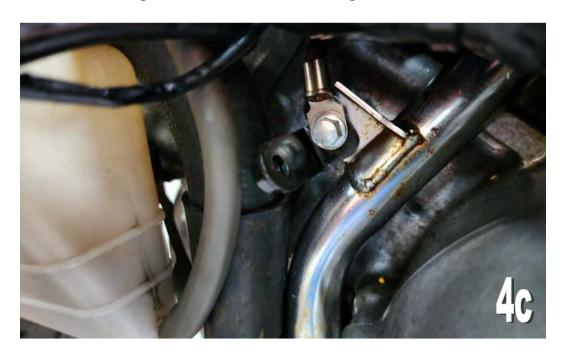
Now fit the coil to the stay as shown using the original bolt. Again, just nip it up in a position similar to shown.
