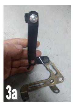
It is easiest to fit the stay to the bike without the coolant tank fitted. The stay fits to the engine mount by way of an M10 bolt.
