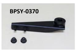
Remove the engine hanger bolt that also retains the rear side of the mid stay and offer up the BPSY-0370 stay between the inside of the lower frame spar and the engine block. The engine hanger bolt then goes through the mid stay, the frame, the bush welded to the BPSY-0370 stay and finally into the engine block.
