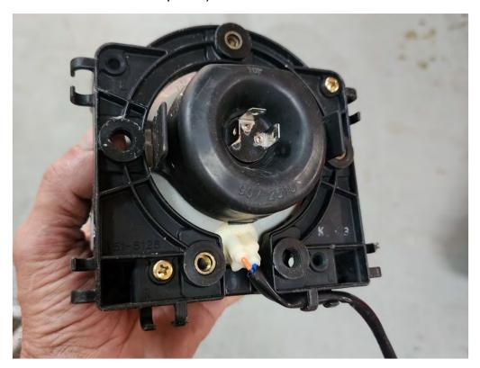
Now, flip the headlight around and fit the headlight rubber shield. Again, you may not have these, so we made our own and are also available on our website. <a href="BPAC-0016 Rubber">BPAC-0016 Rubber</a> Shield, Head Light, Pair, NC30, NC29, MC22 are exactly what you need.
