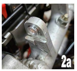
Fit TYLY-0347(W) Tank Mount Rear, RC36-2, RC30 Style (No Fittings) as shown with the bolts provided. Note the direction arrow. This should point to the front of the bike. Try to get the rotation close to the position shown so that minimal adjustment is required when fitting the tank.
