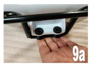
Place the tank onto the frame and rear mount and line up the holes.
