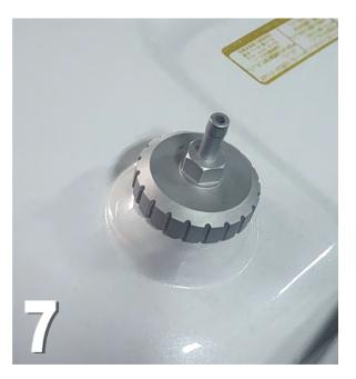
**8)** Fit your choice of fuel filler cap. Either your original R36-2 cap or TYLY-1222 Tank Filler Cap, Keyless, Racing Type, Honda, Type 4
