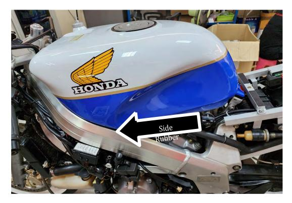
Then fit the tank again and bolt securely into position.
