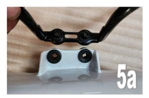
Now fit BPSY-0344 Rubber, Rear Mount, Tank, RC30 and BPSY-0346 Bush, Rear Mount, Tank to the rear of the fuel tank.
