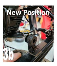
4) Now fit the oil cooler to the bracket using the original RC36 bolt and nut.
