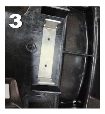
**4)** Now, drill one hole, and physically locate the ECU stay with a bolt (or rivet) so that you can check that it's going to plan so far.
