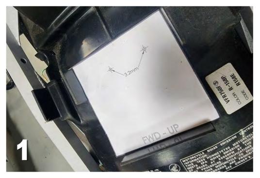
2) With the template in position, use a sharp point to make a mark in the plastic. I used my carbide scriber, but just about anything sharp and pointy will do.
