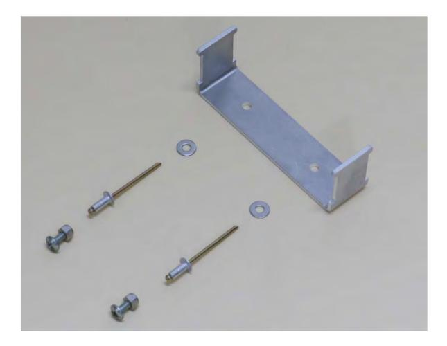
To mount the TYLY-0314X ECU stay, it is required that you drill a couple of small holes in the under tray and secure using either the supplied M3x12 bolts or the rivets. Tools required are a 3.2mm drill bit (not supplied) and a regular electric/battery drill.
