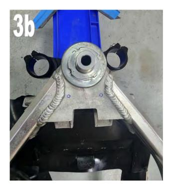
**4)** Now, you can actually set up the rear tank mount (in the TYBP-0009 kit) fairly accurately, based on the marked holes on the head stock. Make sure that the tank is sitting comfortably and no pushing/pulling is required to line up the holes. From there, the rear tank mount should be pretty close. You should be able to see down through the grommets on the front tank mount and upper/mirror stay and see the holes that you just marked.
