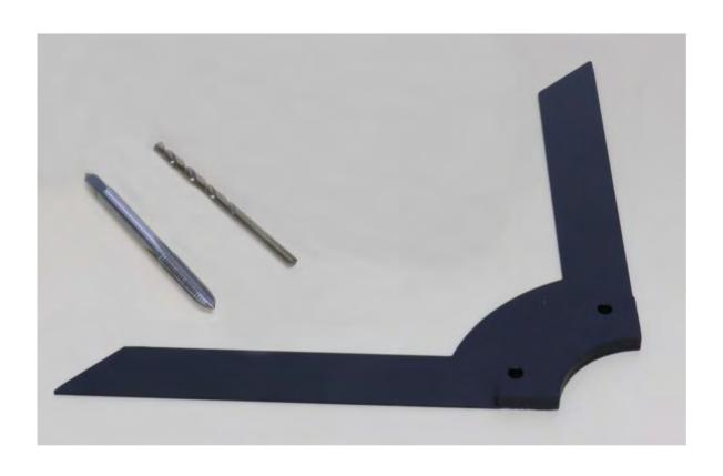
Mounting the BPFG-0009 fuel tank and TYLY-0305 upper/mirror stay on the Honda VFR750F RC36-2 requires that you drill and tap two M6 holes in the headstock area.
