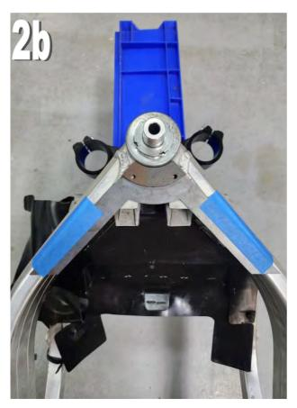
**3)** For a sanity check, mark though the holes with a pen and then remove the jig.
