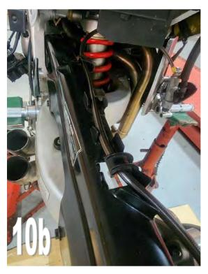
**11)** Adjust the chain tension following the guidelines in the service manual or on the decal on the chain guide. Recommended 20mm. free play. Tighten the pinch bolt to 55Nm.
