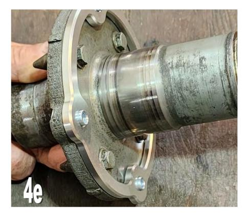
Locate the axle assembly onto the disc and screw in at least one of the M6 bolts to loosely secure the assembly in position.
