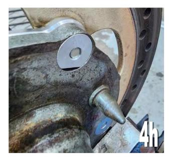
5) Apply grease to the needle bearing in the eccentric, and also a light smear of grease on the axle, and fit the assembled axle into the eccentric.
