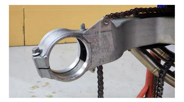
**1)** First job is to fit the stopper TYLY-0326B. This part self locates on the machined step.
