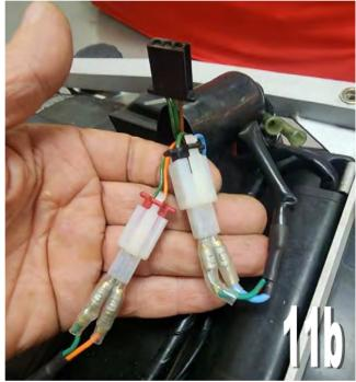
Tuck the wiring away neatly and securely.
