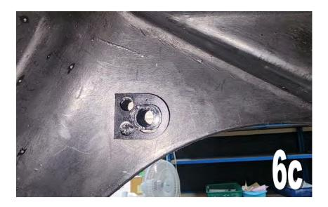
**7)** Now we can thread the turn signal wiring through the hole. Start by offsetting the bullet connectors a little as this will allow easier entry.
