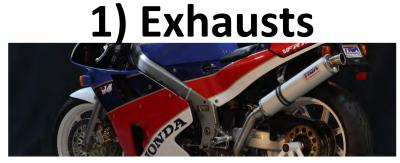
TYGA offer a number of HRC Styled exhausts, so we recommend you take a look at our product range and choose one. Our bodywork is designed to be compatible withthe TYGA exhaust system and is not designed to be compatible with any other exhaust and this may or may not be an issue. Even the stock exhaust, we have not tried fitting because it exits on the right and the RC30 need a left exiting exhaust so why bother?
