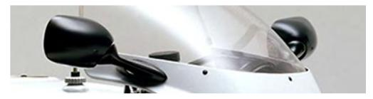
For export models, including Australia, the RC30 had white rectangular mirrors, also with a 40 mm. pitch. This means that the mirrors are completely interchangeable between RC30 models and either type can be installed on any RC30.
