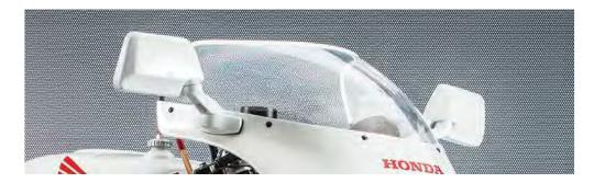
If you don't mind a smaller design, you can install the JDM mirrors fitted to the 250s and 400s at the time.
