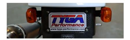
We have designed our fairing to use the JDM turn signals as installed on the RC30 and the early 1989 NC30. Alternatively, the mounting and bullet connectors are identical to other later JDM models that were launched in the 1990s and these bigger ones are easier to source either used or new reproduction so this type is an attractive choice though they are strictly speaking not the correct shape.
