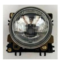
Now, to install them you will need bulbs, running lights and rubber boots. We have limited supply of rubber boots used and will source new ones so we should be ok there. You can also at a pinch use the boots off the VFR750F headlights. However, they are a bit too big and may not seal that well.
