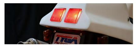
Honda again raided the part bin for the taillight so we are in luck in that the NC30 taillight is the same shape and almost identical to the RC30 one.
