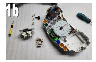
2) The electronic module is simply clipped onto the back of the speedo and is removable without tools. There's a couple of little plastic clips, but they can be easy pressed out of the way to remove the module.
