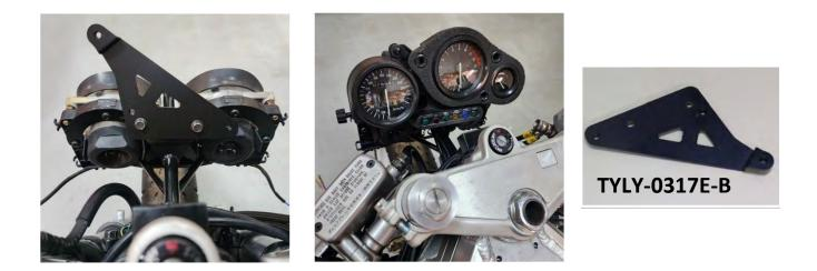
A second choice is the meter assembly from the '92-'93 CBR900RR SC28 . This is closer in looks to the RC30 meter thanks to the arrangement of the warning lights. One issue here though is that the speedo is mechanical drive as the early SC28 takes the drive directly from the front wheel.
