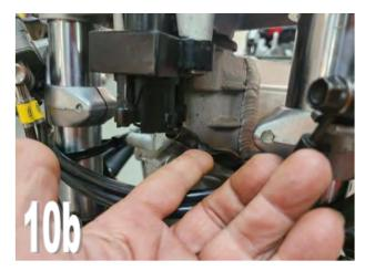
**11)** Route the ignition switch wire on the left side of the fame and connect the plugs as shown
