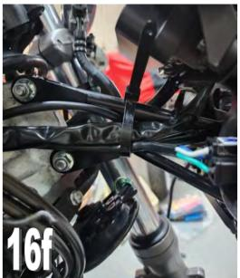
The running light and turn signal wires run over the top of the headlights and down the outer edges. There are hooks on the headlights to retain the wires.
