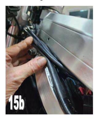
The extension harness runs on the underside of the lower frame spar.
