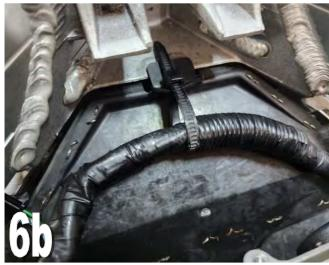
**7)** Now hold the harness as shown, and at an approximate point between the headlight connectors and headlight relay, fold the harness back on itself, and secure the bend with a cable tie.
