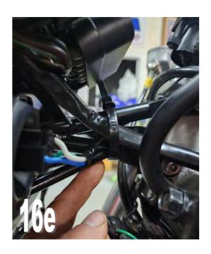
The wires for the running lights and turn signals should route through the meter stay behind the meter, and then split left and right.
