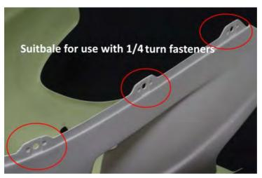
However, for these instructions, we are using the M6 clips. So fit the 6x M6 clips to the mounting tabs.
