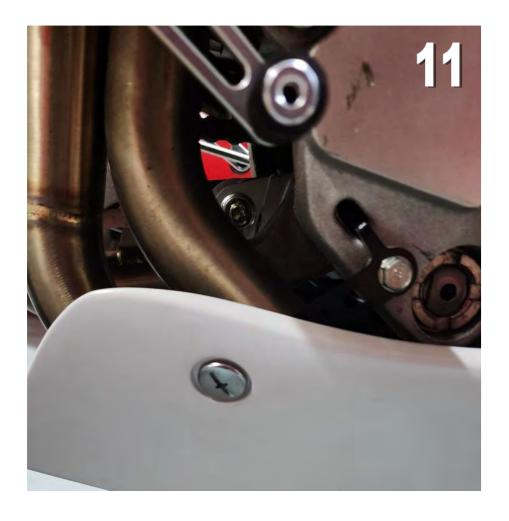
**12)** Fit the bodywork bolt and plastic washer to the lower left stay.
